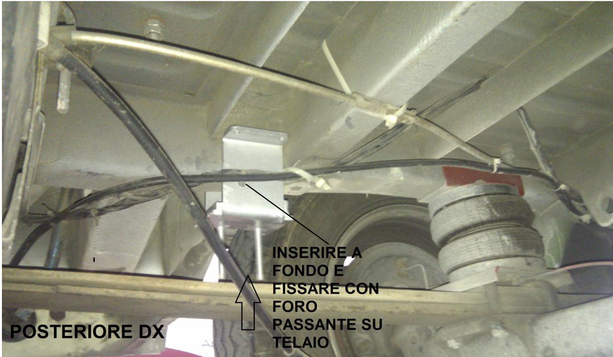
The adapter must be placed in front of the rear axle, in the points shown.
