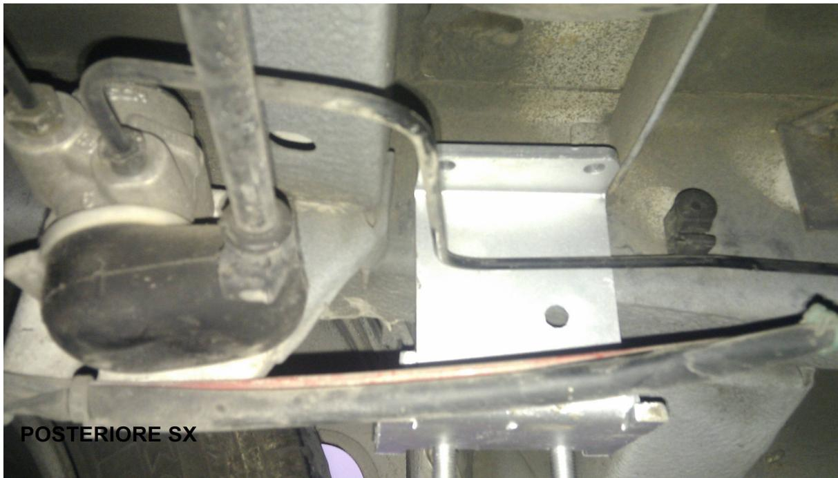
Insert the adapters then drill the 10mm holes (on both sides) – Then insert and fit the connection bar.
