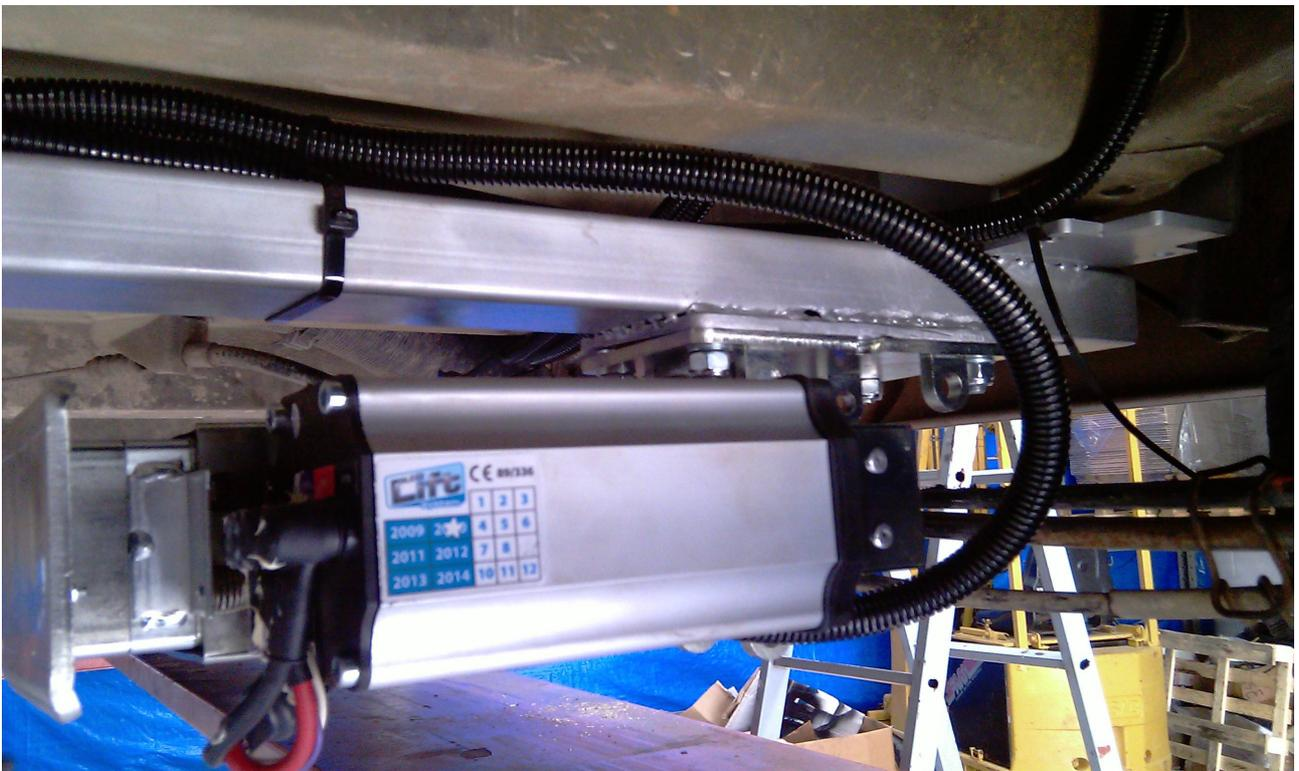
**BOTH JACKS MUST BE FIT WITH THE ENGINE REAR AND ROTATION INSIDE THE VEHICLE.**
