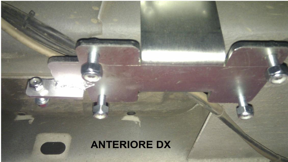
Put the adapter on the chassis, under the cabin's door.
