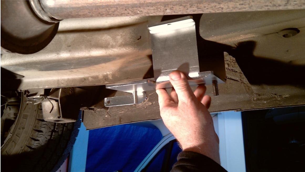
Put the adapter most rear possible, if necessary remove any sealing material for a perfect adherence, use a bottle jack to stop the bracket in the correct position and make the 8mm side hole then fix with the bolt.
