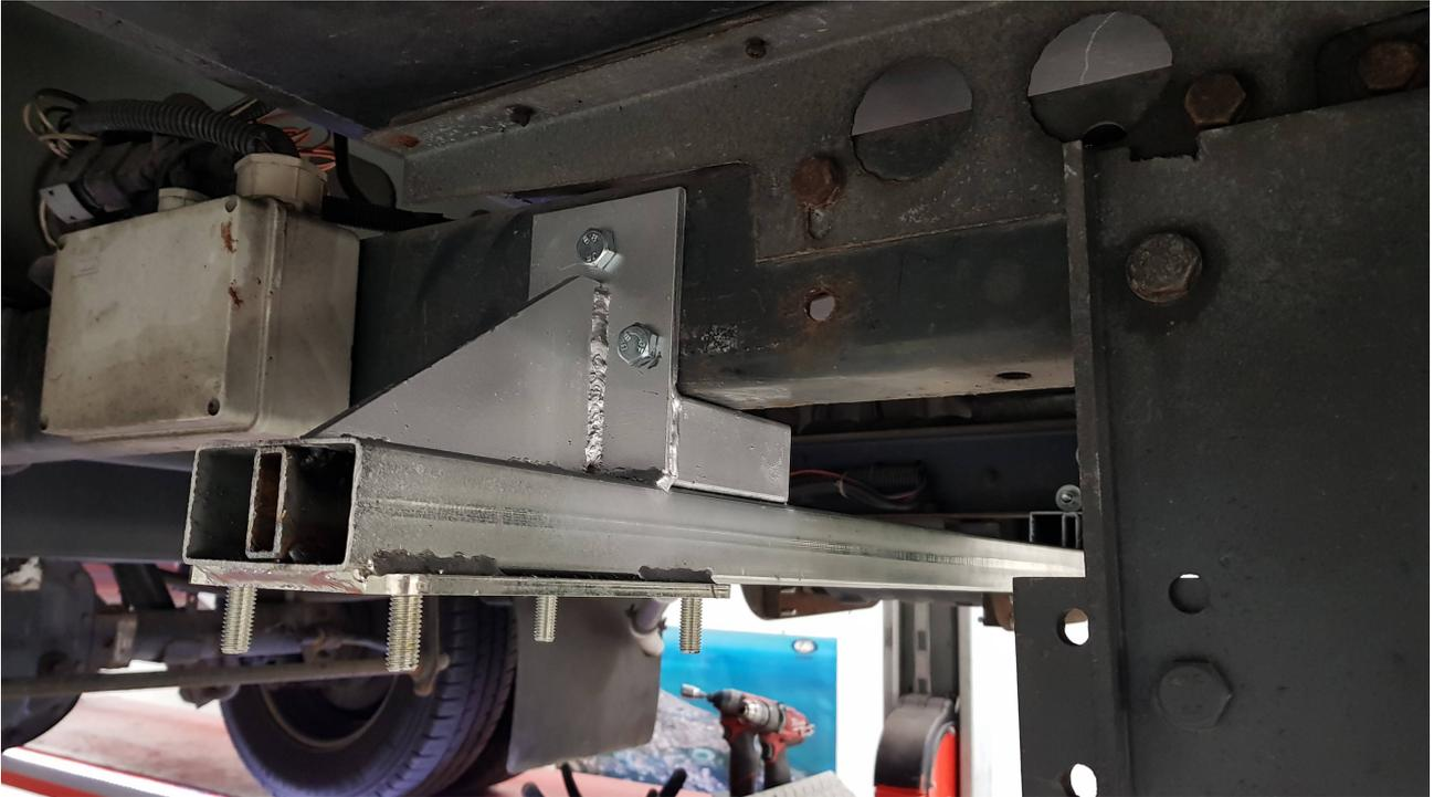
Put the adapter rear the rear axle, be carefull that the adapter is completely insert before drill the holes, is some case is possible to use holes already present on the chassis.
