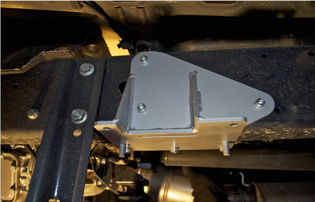
The adapter must be placed just behind the gearbox cradle and is fixed using the three M8 screws supplied, without drilling any holes on the frame if the frame is of the latest model (BLACK) otherwise drill the 3 holes.
