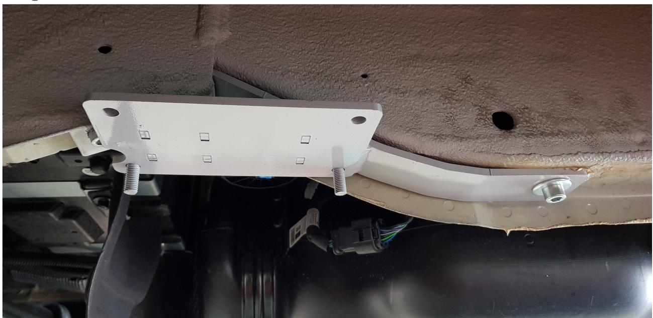
Fit the adapter with the bolts supplied
