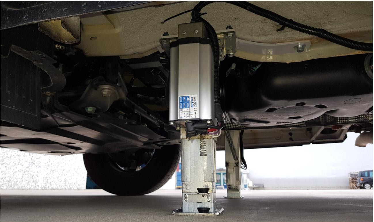
***EXAMPLES OF JACKS CORRECTLY INSTALLED***
