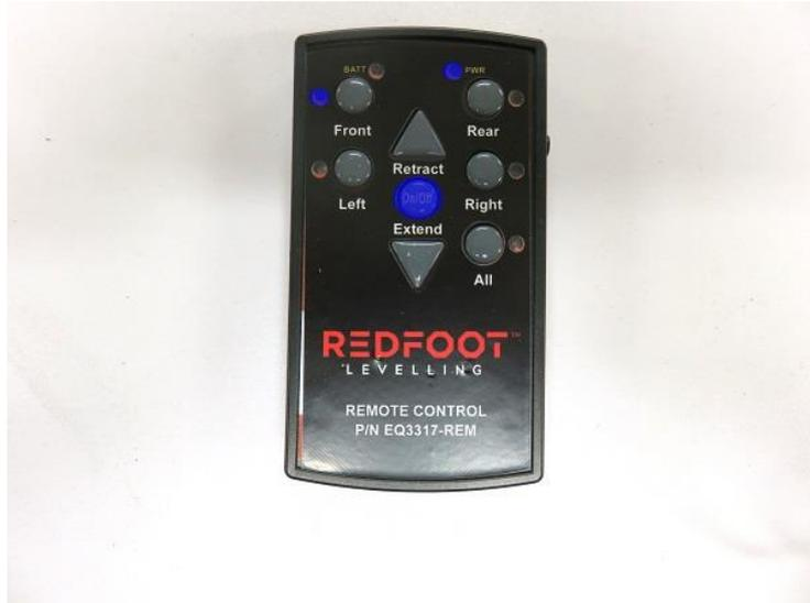
Push the “Extend” button, the power light should flicker to indicate it is signalling and pairing to the Controller Board and the corresponding cylinders should now be travelling in a downward direction. You will hear the pump operating; it is important to verify the legs are planted on to the ground securely.
