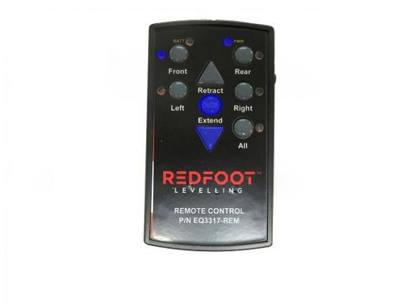
Continue operating the Wireless Remote-Control Keypad by ‘Extending’ or ‘Retracting’
