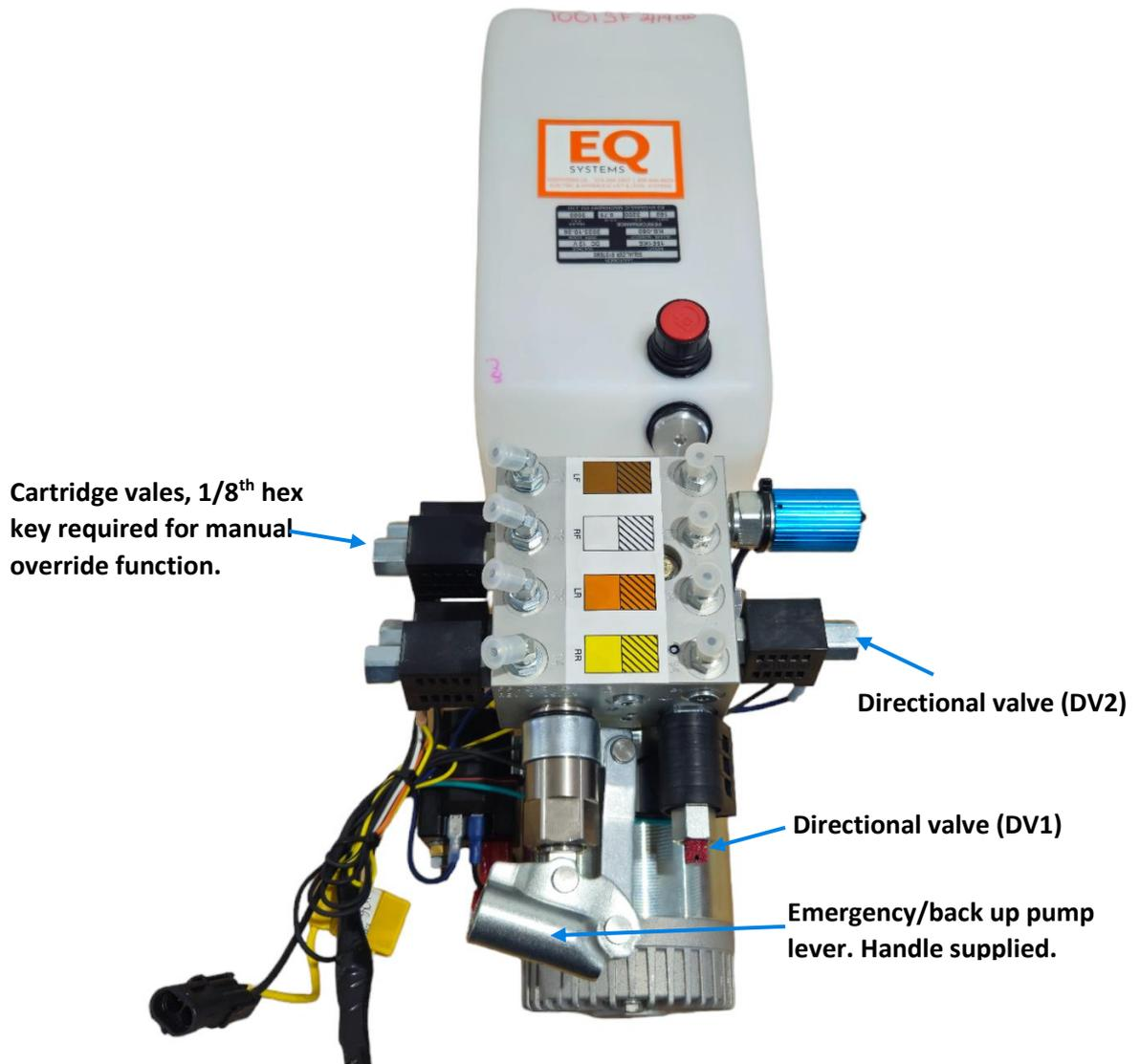
On the 7001 SF Pump the return and extend connections banks are on the opposite side to the standard 784X KS pumps. As seen in the diagram above, the return banks (striped box) are on the right side of the pump manifold and the extend (solid colour) banks are on the left side of the pump manifold.
