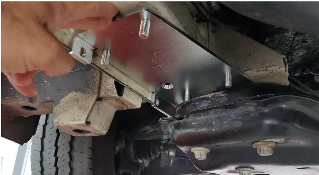
5. Fix the adapter to the special plate that you insert into the hole.
