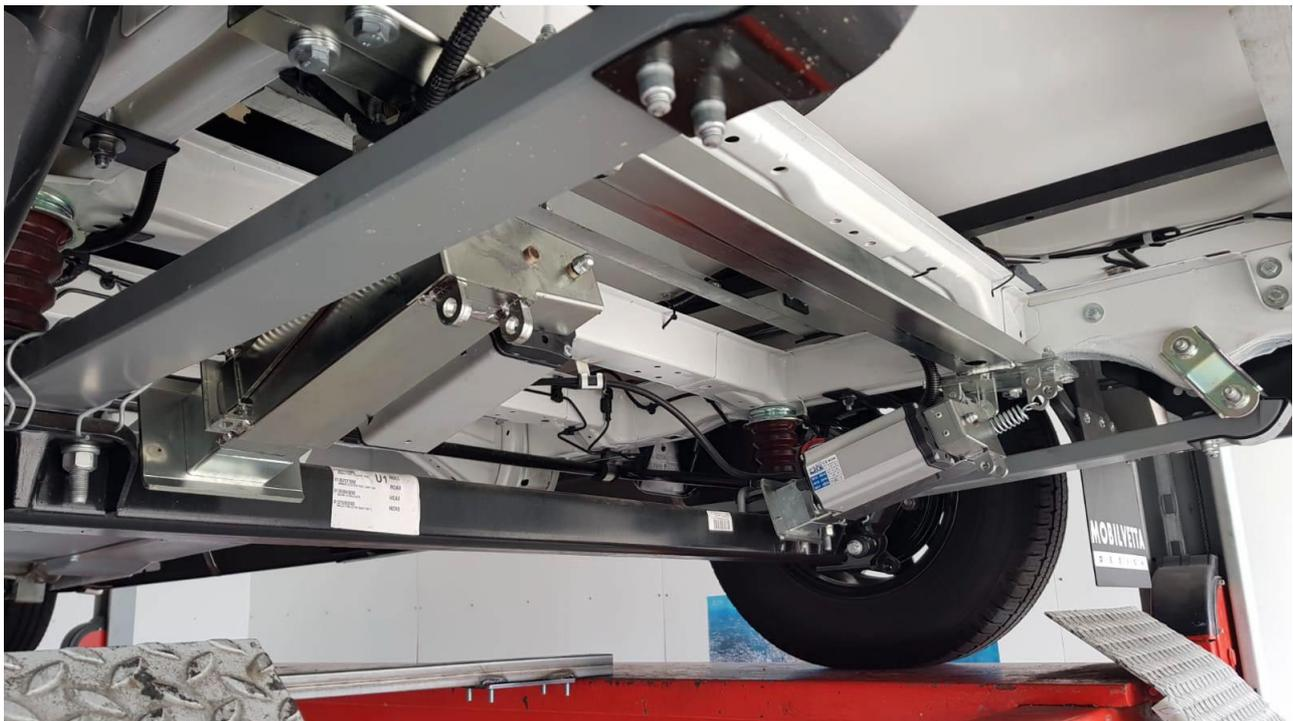
**BOTH REAR JACKS WITH ENGINE TO THE INSIDE OF THE VEHICLE AND ROTATION IN FRONT OR REAR**
