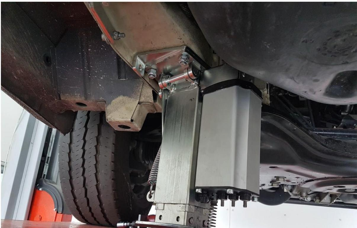
The above image shows the jack with the motor to the inside of the vehicle and rotated to the rear.
