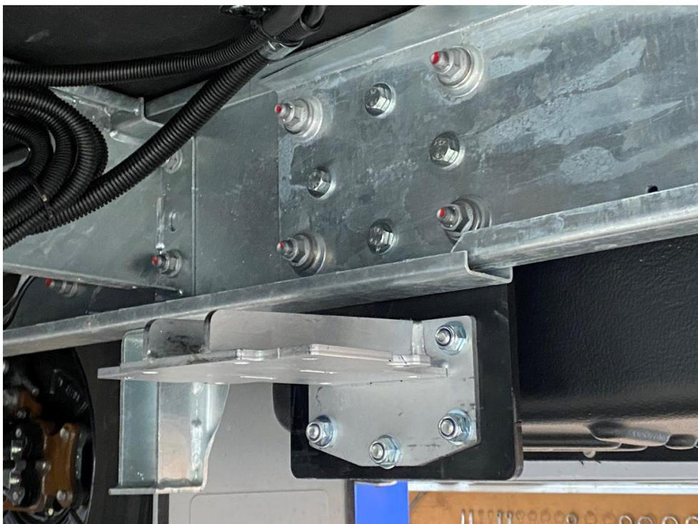
Install the two cross braces supplied on the top of the jack bracing bracket as shown using the four longer 10mm bolts.
