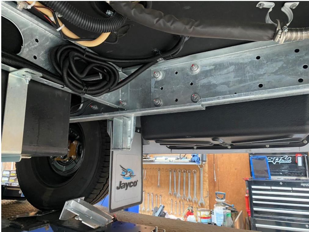
Use the bolts/nuts/washers provided to mount to the outside of chassis.
