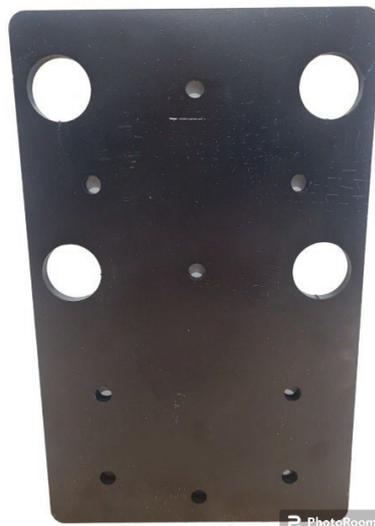
Using the mount plate as a template, mark and drill four 10mm holes at the chassis extension point as shown. The mounting plate is designed to mount over the outside of the chassis four extension bolts.
