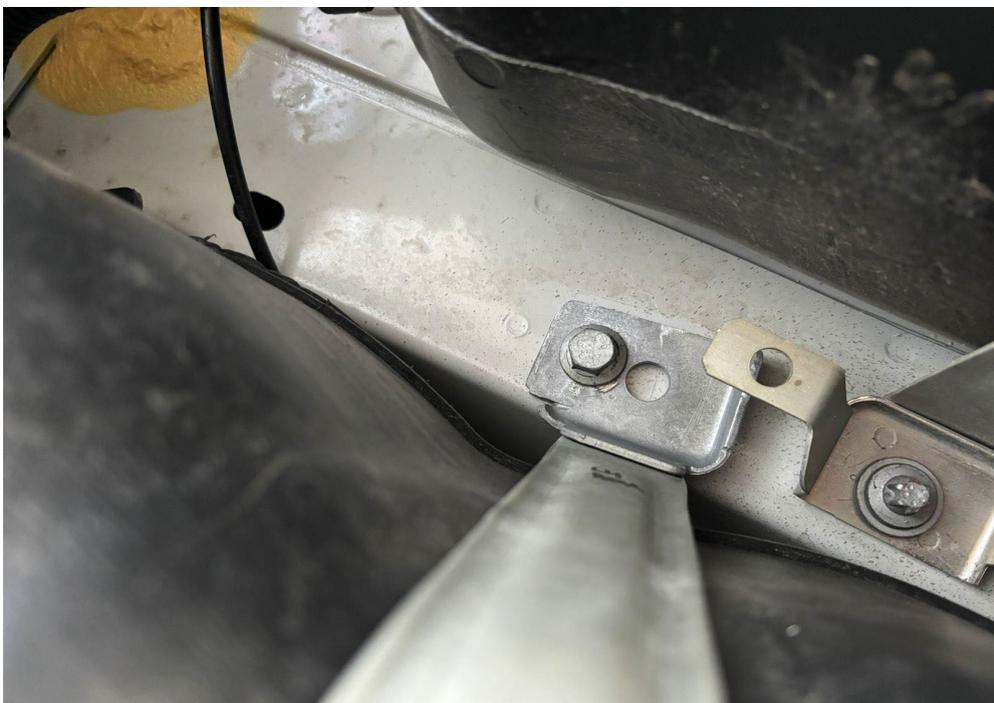
Rounding of the passenger side front left hole to 12mm.
