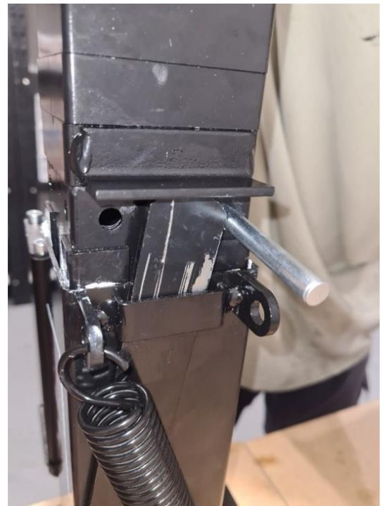
Step 4. INSERTING PINS - Be mindful not to use excessive force putting the pin back in. This can cause damage and not allow the circlip to reseat. If it doesn't slide through take it out and drill hole to no more than 9.5mm a hole.
