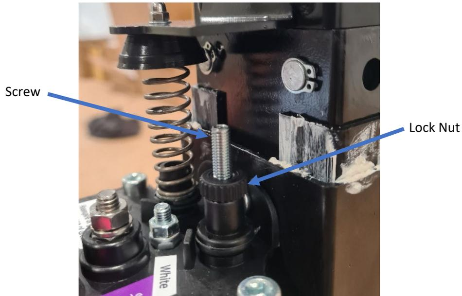
The limit switches must touch before the mechanical end point of the jack. Leave enough clearance between the cut-off point of the limit switches and the mechanical stop of the jack to compensate for moments of inertia. There needs to be at least 1cm of play up to the mechanical stop from the limit switch. If the limit switches are not adjusted correctly most of the functions will be blocked. If unsure, call Redfoot Levelling for assistance on 07 5228 0211.
