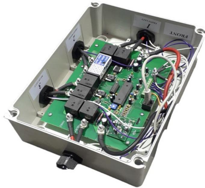
Ensure the control box label 'FRONT' is closest to the front of Van. The box must be mounted flat to the floor underside.
