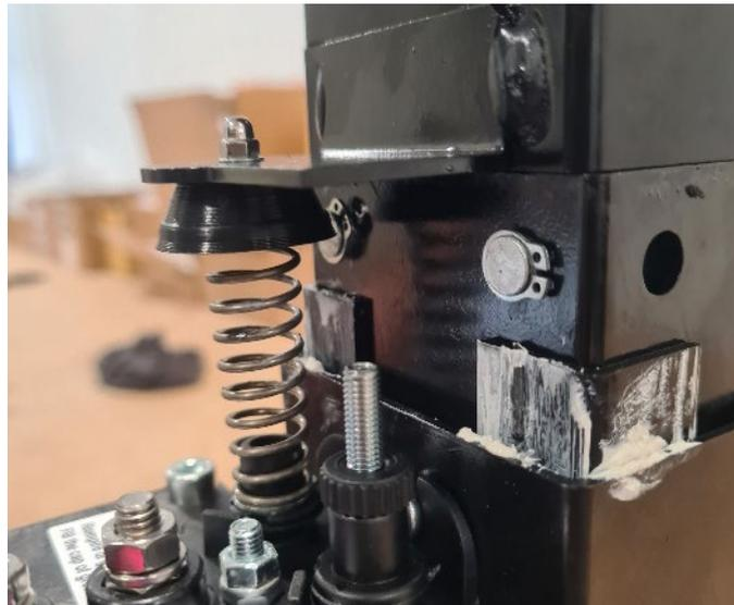
**Note:** Each kit comes with enough spacers to add a maximum of 120mm extension to each jack leg stem. There are 3 sizes, 10mm, 20mm and 40mm. Remember the pressure switch/push bar plate is 20mm.
