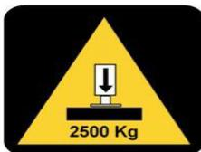
**Use fixing points with sufficient stability. Consider every jack can lift to 2500 kg. If necessary, the fixing points at the chassis must reinforced with adequate parts.**
