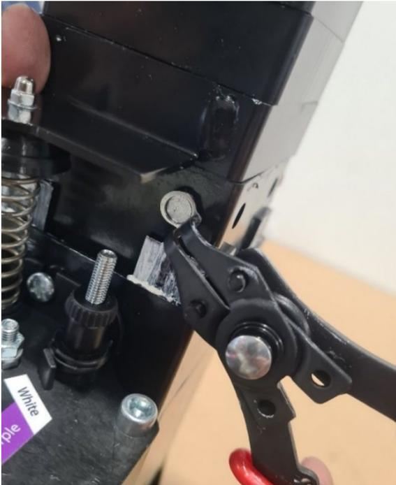
Step 1. REMOVE JACK STEMS - Using circlip pliers carefully remove the circlips without stretching the circlip too much. It is best to come from the side closest to the motor and push the circlips out.
