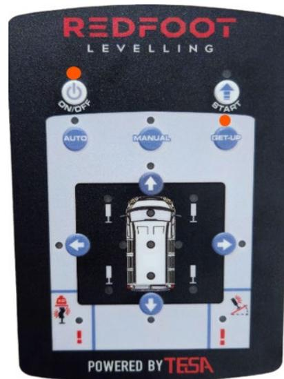
The panel will display a status light or lights in the middle of panel. These status lights will display the lowest ground point underneath the van. The status lights will change depending on the slope and position of the van. The green light will illuminate once you have achieved level.
