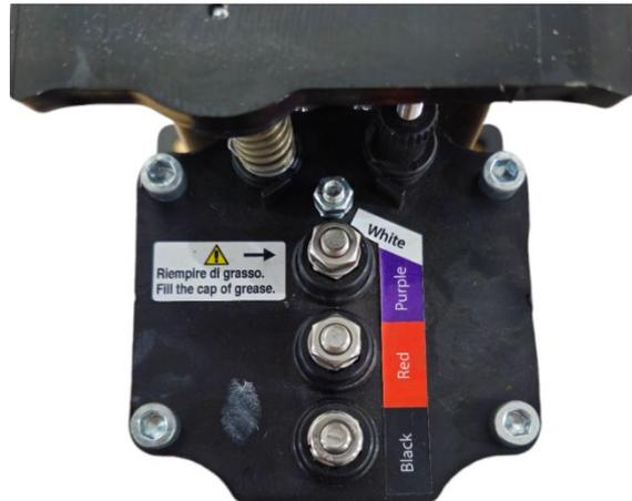
After fitting (purple cable only) make sure to fill the rubber cap with the supplied grease. Do not grease or fit rubber cap before securing cables to avoid grease affecting contact with the post. The grease avoids accidental ground with other connections caused by splashes of water and/or debris.
