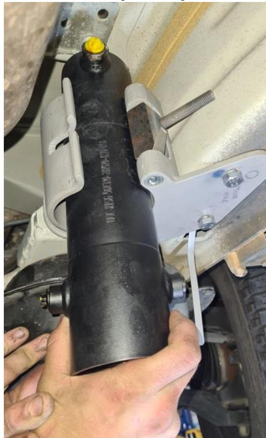
**Place the Clamping Bar over the existing pivot bolt as shown and attach the M10 Nyloc nut.**
