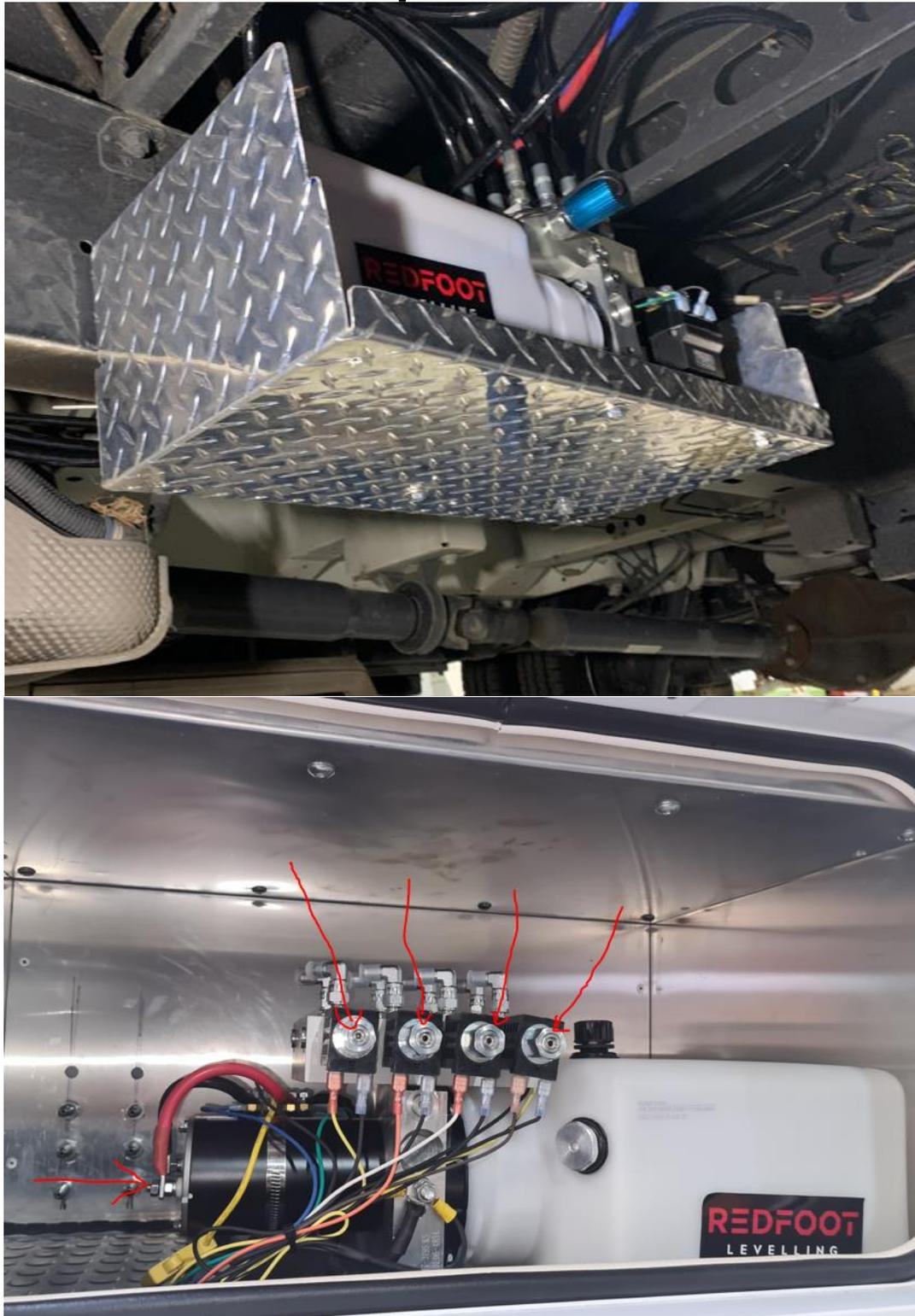
The ideal location for the Pump/Manifold can be inside E.g Storage compartment or outside the vehicle as shown. The important thing is to have ease of access in the case of a 'manual override' to retract all cylinders. This can only happen if you lose all power to the system and you need to move on from your site.
