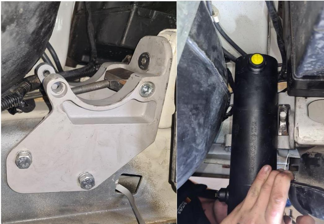
**Hold the cylinder in place and use the Clamp Plate to align with the bracket holes, insert the M10 100mm Socket Head Screw bolt as shown.**
