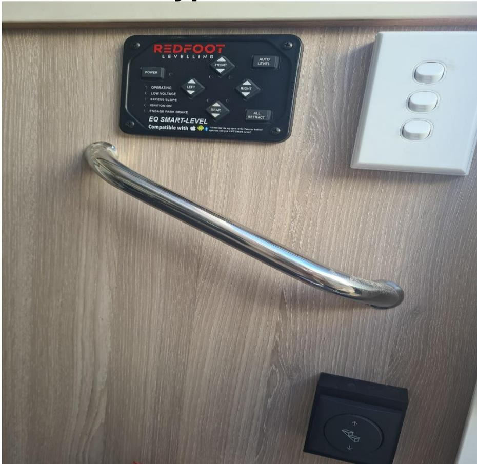
The ideal location for the keypad is near the entrance inside the vehicle. For ease of use, mount the keypad on the side as you enter the motorhome so when you are facing the keypad you are facing forward in the vehicle. (Like you are driving the vehicle)
