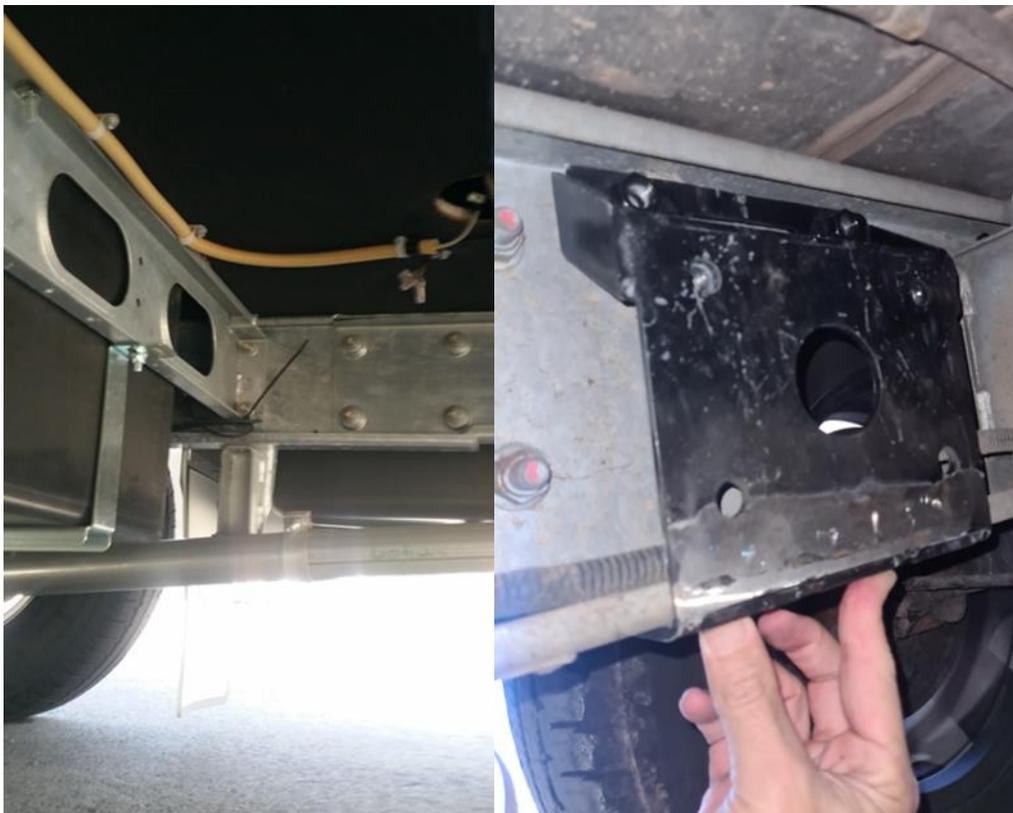
37. The location for the rear brackets is to be mounted flat against the inside of the chassis rail, within 100cm behind the rear axle. Finding free real estate in this area is key.
