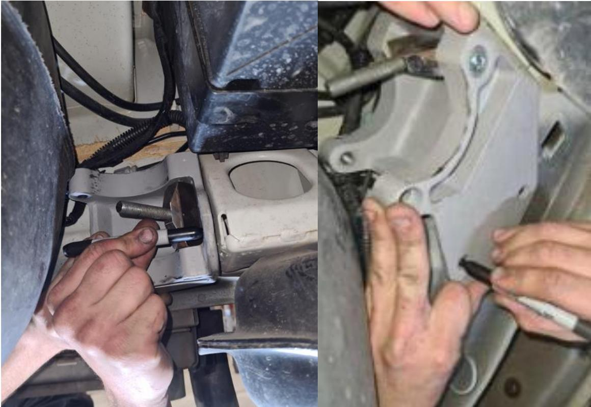
**Drill through chassis as marked**
