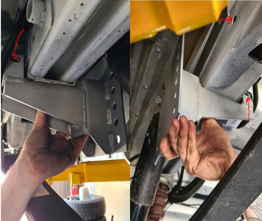
**Arrows point to the locations to bolt onto the chassis**
